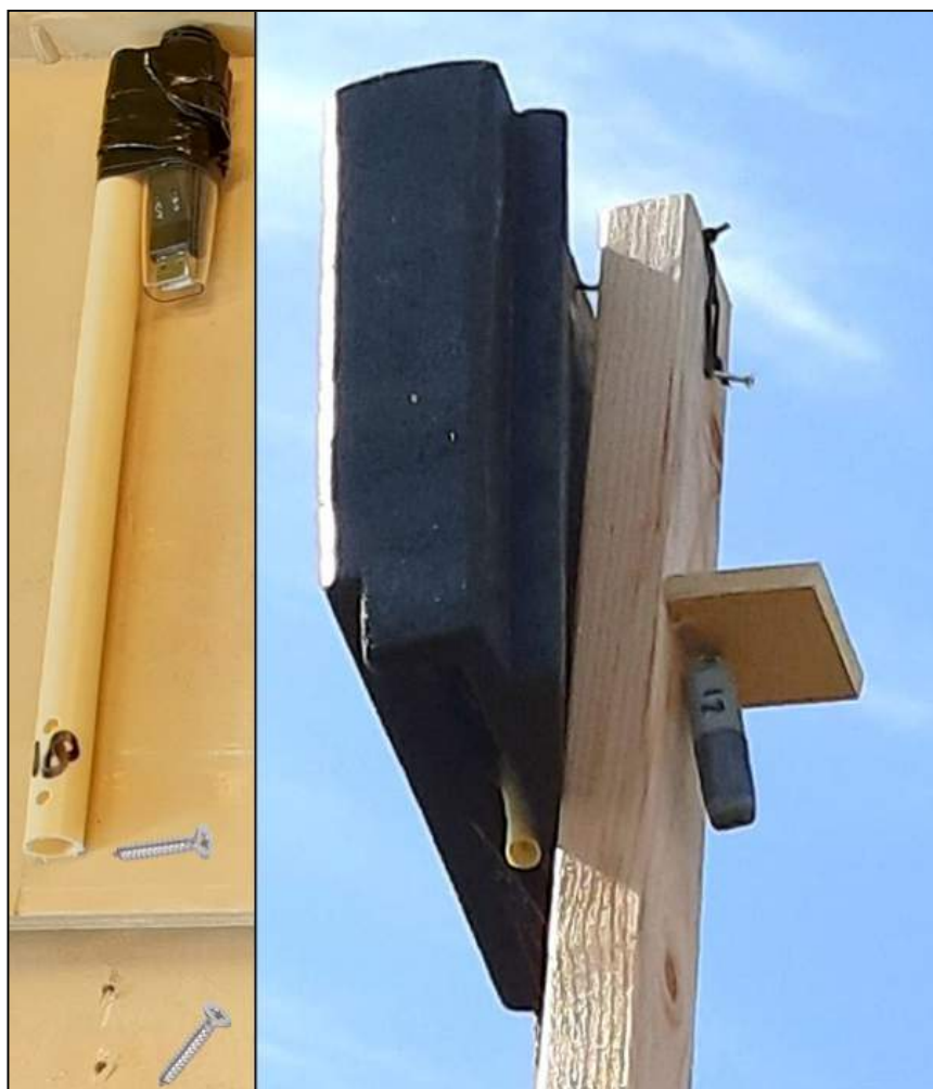
Figure 3 Each PVC dowel with logger was incorporated in the bat box and was mounted to the bat boxes with screws (left). To measure ambient microclimate, each cluster was provided with a north-facing data logger attached to one of the middle bat boxes (right).
